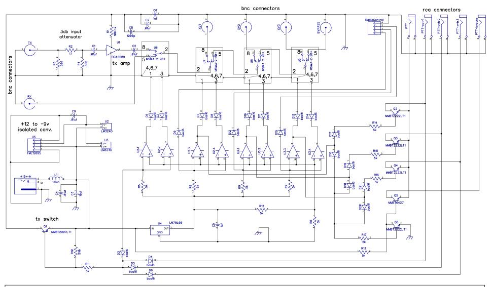
receiver attenuation measured .6db for xv1, 1.1 for xv2, 1.5 for xv3 and 1.9 for bypass. with a 3db input attenuator value, transmit gain from 1 to 200 MHz was 18db with 1db gain compression at +15 dbm. At +10 dbm, there was no measureable gain compression. From 400 to 1400 MHz, transmit gain varied from 16.5db to 12 db, and gain compression readings were the same as measured from 1-200MHz. Isolation between xv1, 2 and 3 was in excess of 50db to 200 MHz, and greater than 35db at 1400 Mhz.
