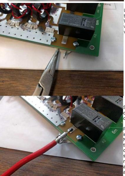
Using a pair of needle-nose pliers, bend the ends of the lugs vertical as shown. With the lugs formed in this way, there will be considerable strength in both the vertical and horizontal planes.
