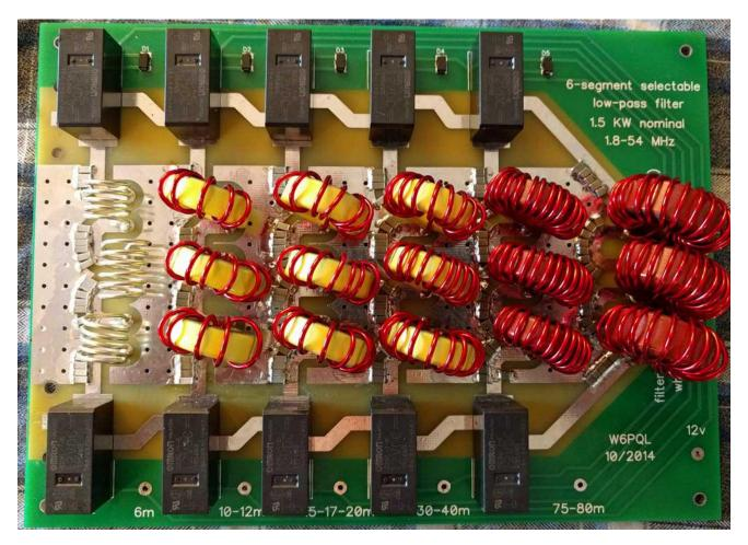
Note: If using this filter for the W6PQL single amplifier pallet, 3<sup>rd</sup> harmonic levels returned to the rf deck by this type of filter can be 100 watts or more at 1kw output, and will interfere with proper operation. Optimum performance is achieved with a stand-off cable length of 34 inches; this is the recommended total coax length from the output of the rf deck to the input of the filter, and will minimize the interference caused by reflected power.
