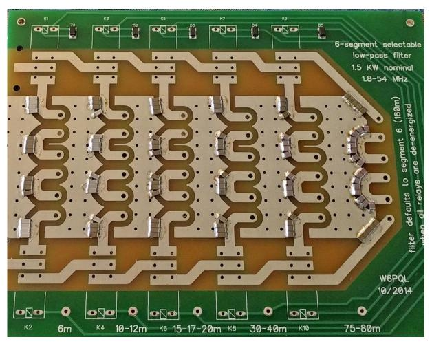
On the back side of the PCB nearest the 6m section, the 5pf capacitors are installed as shown. Solder only the ground plane side of the capacitors (for now) until the relays are installed.
