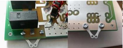
Secure two solder lugs as shown here using the 4-40 machine screws provided; leftmost photo is top side, rightmost photo shows the two locking nuts on the other side securing the lugs.
