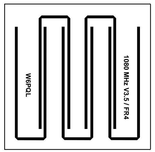
gaps = .024 and .036 tap at 12mm from center cf = 1085 MHz IL = 5.8 db +- 50 MHz = .8/5.5 +- 100 MHz = 14/26 +- 150 MHz = 32/38
